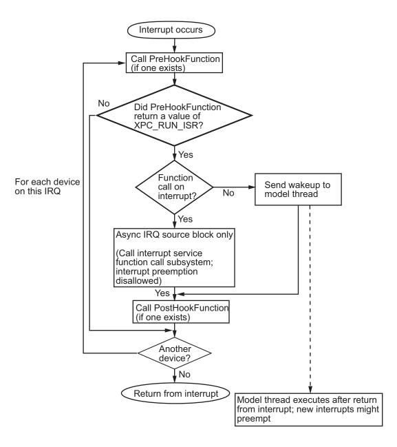
When a hardware interrupt occurs, the generated code uses the following steps for each device on this IRQ to determine which device generated the interrupt:
